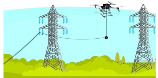
Drone performing transmission line work.
